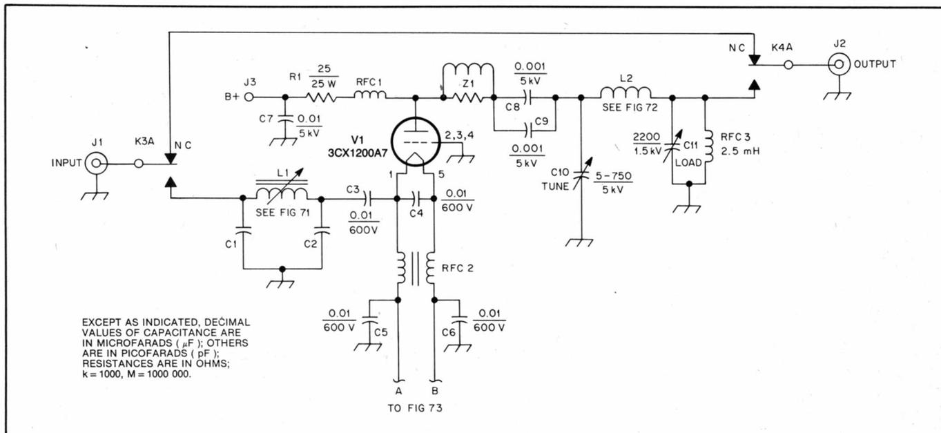
Fig 70—Schematic diagram of the 3CX1200A7 amplifier RF deck. Details of the input and plate-tank circuits are shown in Figs 71 and 72.
