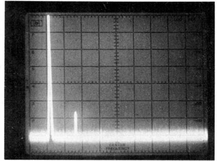
Fig 78—Spectral photograph of the 3CX1200A7 amplifier operating through the low-pass filter. Power output is 1500 W at 14 MHz. Each horizontal division is 10 MHz; each vertical division is 10 dB. All harmonics and spurious emissions are at least 56 dB below peak output.
