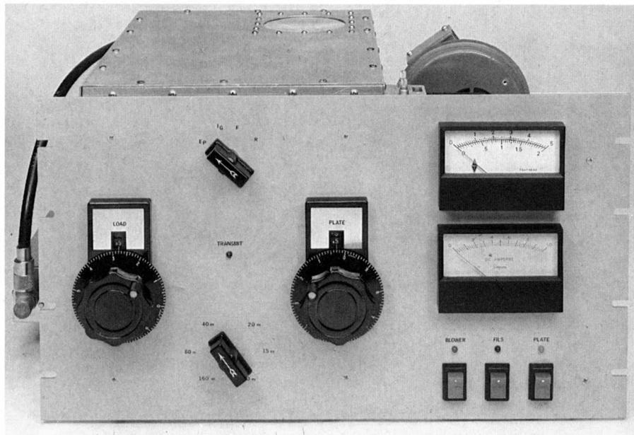
Fig 69—The 3CX1200A7 160- to 10-meter amplifier is built behind a standard 19  $\times$  10½-inch rack panel. Vernier drives are used to control the loading and tuning capacitors. The top meter can be switched to read plate voltage, grid current, forward power and reflected power. (The meter switch is above the LOAD and PLATE dial drives.) The bottom meter is dedicated to plate current. An external low-pass filter is mounted on the left side of the chassis.
