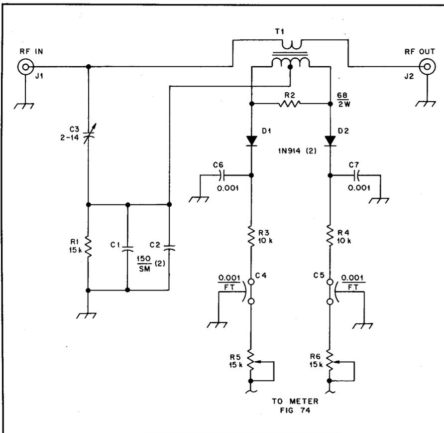
Fig 75—Schematic of the wattmeter circuitry for the 3CX1200A7 amplifier.
