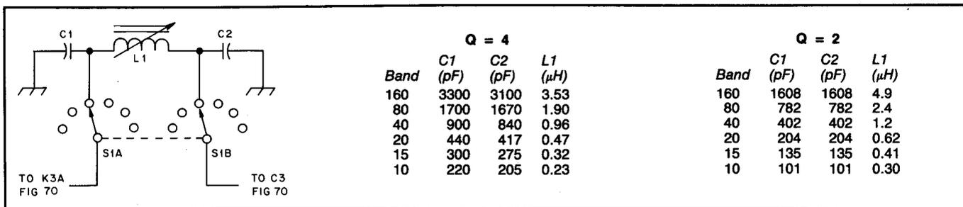
Fig 71—Details of the 3CX1200A7 amplifier input circuit. Component values are shown for Q = 4 and Q = 2. The amplifier was built using the values for Q = 4 (see text).
