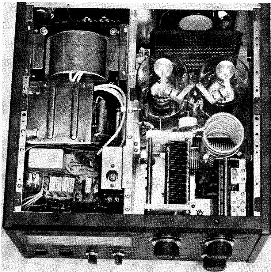
Fig. 1 — An interior view of the Kenwood TL-922A linear amplifier. In the power-supply compartment on the left, the massive high-voltage transformer is visible at the rear. A second transformer, which supplies filament, relay and lamp voltages, is located under the circuit board at the front.
